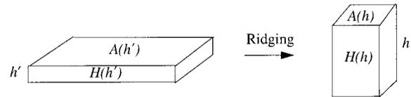
FIG. 1. Illustration of how thin ice of thickness  $h'$ , area  $A(h')$ , and enthalpy per unit area  $H(h')$  is transferred into thicker ice of thickness  $h$ , area  $A(h)$ , and enthalpy per unit area  $H(h)$  owing to ridging.
