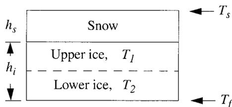
FIG. 3. Schematic representation of the Winton (2000) three-layer thermodynamic model. For each ice thickness category  $h_i$ , the model computes snow thickness  $h_s$ , upper ice temperature  $T_1$ , lower ice temperature  $T_2$ , and ice growth rate  $f$ . The temperature at the bottom of the ice is fixed at  $T_f = -1.96$ , the freezing temperature of seawater. The temperature at the surface of the ice or snow,  $T_s$ , is determined from a surface energy balance.
