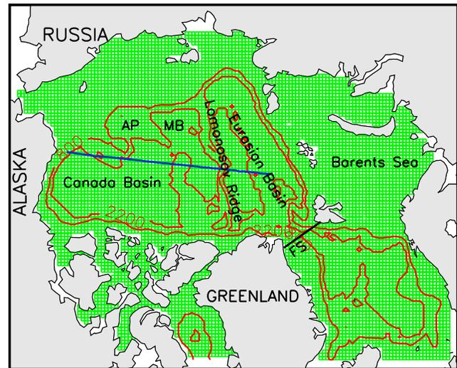
**Figure 1.** Model grid configuration (40-km horizontal resolution illustrated by green lines), and bathymetry (red contours with the interval being 1400 m). The blue line between Barrow, Alaska and a location in the Eurasian Basin represents part of the SCICEX cruise track in the fall of 2000 along which CTD measurements are available. Fram Strait (represented by the black line), Arlis Plateau, and Makarov Basin are marked as FS, AP, and MB.
